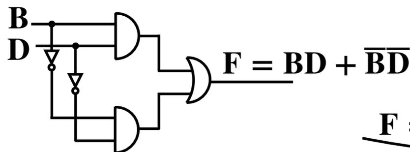
$F = \overline{\overline{F}} = \overline{\overline{BD + \overline{B}\overline{D}}}$
